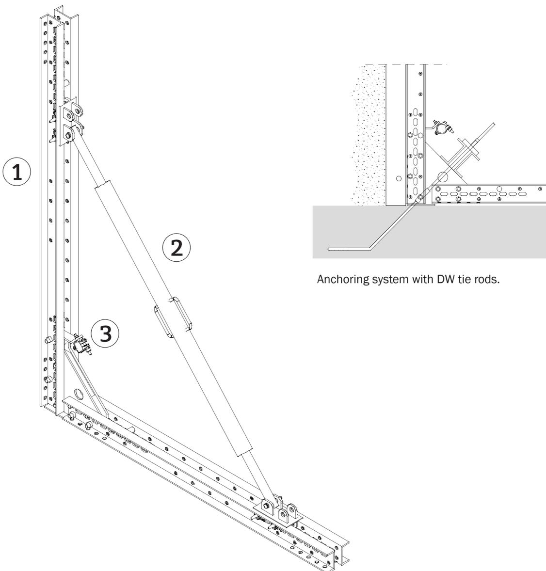
Anchoring system with DW tie rods.
